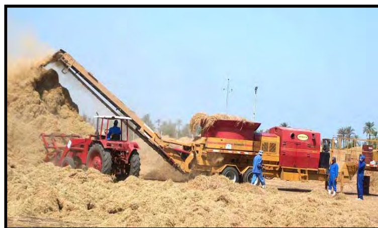
Picture no. (24): Design and construction units for producing compost from agriculture residue (rice straw)
