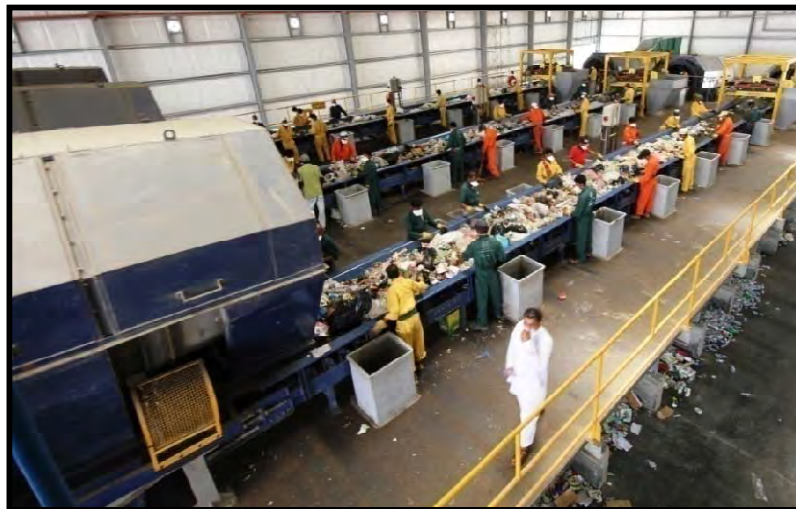
Picture no. (15): Seder municipal solid waste sorting and recycling plant – Jeddah KSA
