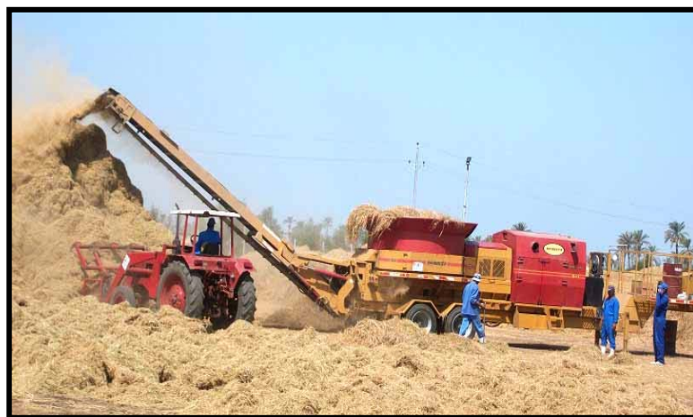
Picture no. (30): Design and construction units for producing compost from agriculture residue (rice straw)
